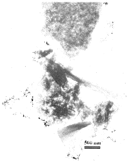
Fig. 6-1 TEM image of freeze-dried Halocynthia cellulose with sulfuric acid impregnation, carbonized at 600°C.
