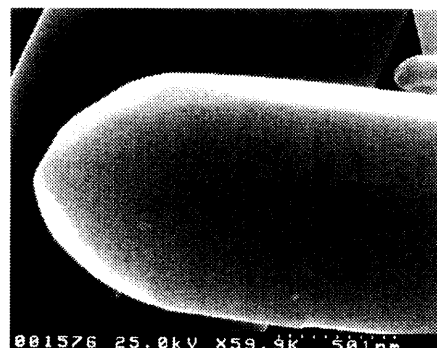
Fig.3 Elongated photograph of tip portion of whisker grown with \text{In}^{3+} as impurity.
