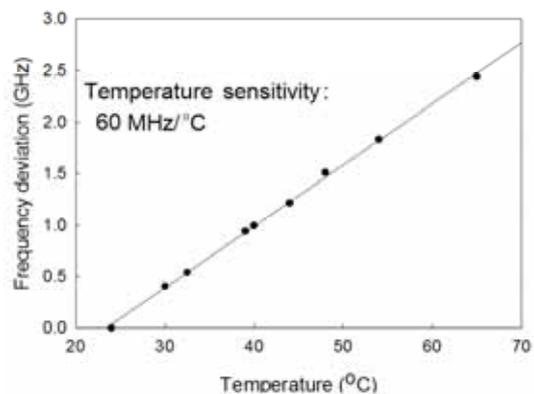
Fig. 3. Temperature dependence of Bragg frequency shift of the reflection peak.
