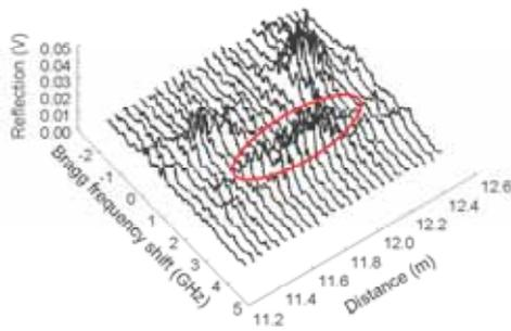
Fig. 4. Reflection spectrum of the dynamic grating localized at strained section.
