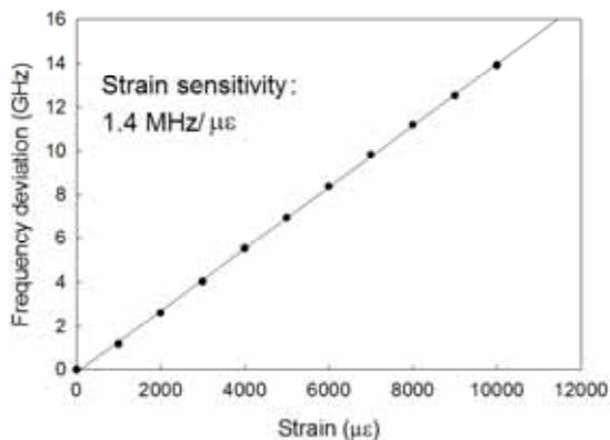
Fig. 2. Strain dependence of Bragg frequency shift of the reflection peak.
