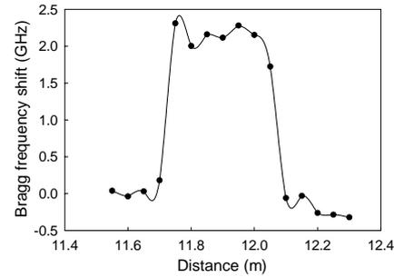
Fig. 5. Bragg frequency shift when sweeping the coherence peak along the fiber.
