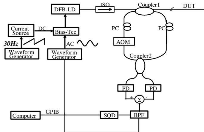
Fig. 6. Experimental setup for high-accuracy high-speed adaptive reflectometry.
