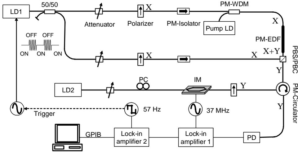
Fig. 1. Experimental setup to detect reflection from dynamic grating in PM-EDF.
