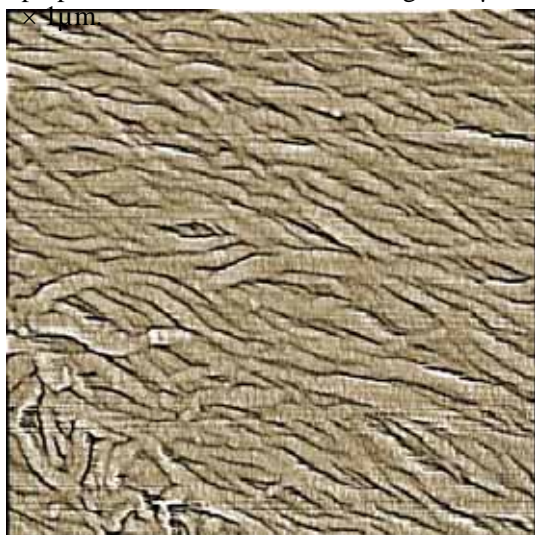
Fig.5 AFM image of a 1/5 metal coated CPD pulp fiber surface in air. The image is 1\mu\text{m} \times 1\mu\text{m} .
