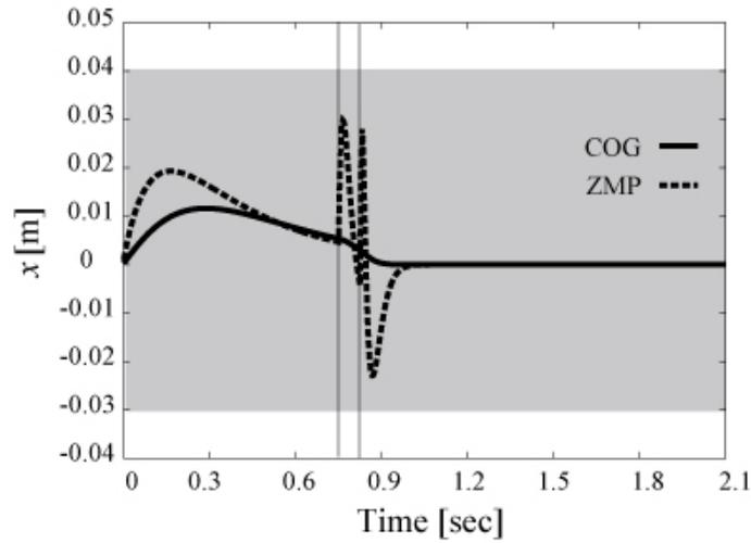
Fig. 7 Initial response of the system when switching control applied. At 0.75[sec] and 0.84[sec], controller switched the compensator.
