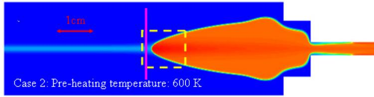
Fig. 6 Instantaneous temperature distribution for PHT : 600 K and PHW : 1mm.
