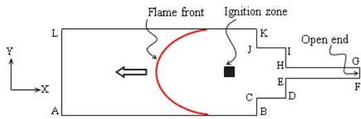
Fig. 1(a) Schematic view of the simulation domain and coordinate system.
