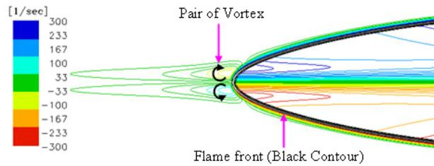
Fig. 8 Visualization of weak pair vortex (by vorticity contour) ahead of flame tip due to negative velocity distribution (shown in Fig. 7)
