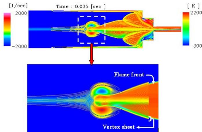
Fig. 9 Visualization of the strong flame-vortex interaction by the temperature (in solid) and vorticity [1/sec] (in contour) distribution for PHT: 600 K and PHW: 0.5 mm.
