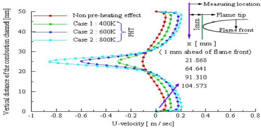
Fig. 7 The detailed negative velocity distribution 1 mm ahead (it is located at the pink-colored vertical line in Fig. 6) of flame tips for pre-heating and non pre-heating effect.
