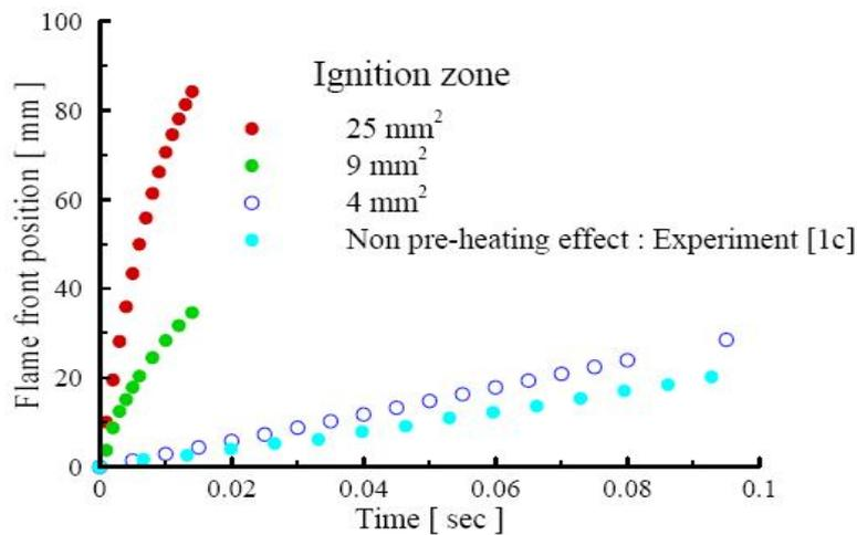
Fig. 4 The flame front location versus time along the center line ( $y = 25 \text{ mm}$ ) of combustion channel.
