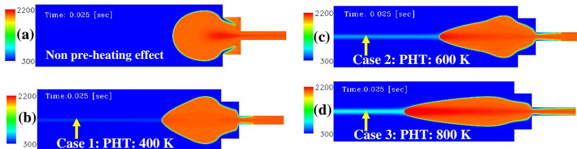
Fig. 5 The temperature distribution in the combustion channel: (a) for non pre-heating effect and (b) for PHT of Case 1, (c) for PHT of Case 2, and (d) for PHT of Case 3 at time 0.025 sec with 1 mm pre-heating width (PHW), (Here, PHT: stands for pre-heating temperature)
