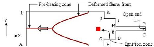
Fig. 1(b) Schematic view of the installation of pre-heating zone in the calculation domain.
