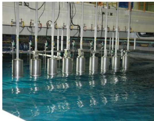
Fig. 2 A Sketch view of the experiment of an array of porous cylinder
