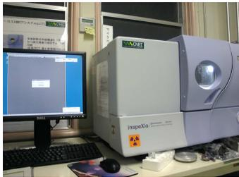
**Figure 7 inspeXio SMX-90CT microCT**
