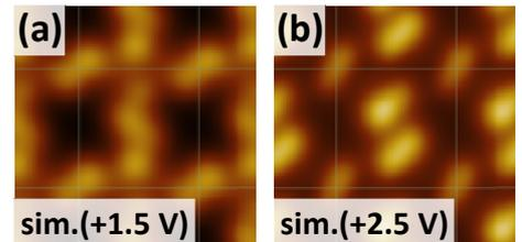
Figure 5: Simulated STM images at (a):  $V_s = +1.5 \text{ V}$  and (b):  $V_s = +2.5 \text{ V}$  based on the proposed model [5].
