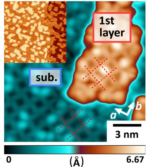
Figure 6: STM image ( $15 \times 15 \text{ nm}^2$ ,  $V_s = +1.5 \text{ V}$ ,  $I_t = 30 \text{ pA}$  at 77 K) taken on the ultrathin STO film with thickness of 0.3 ML. Red broken lines are guides of the  $(\sqrt{13} \times \sqrt{13})$  mesh structure.
