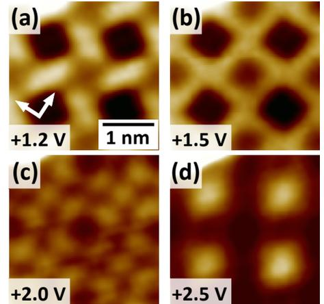
Figure 4: Bias-dependent STM images of the  $\text{STO}(001)-(\sqrt{13} \times \sqrt{13})$  surface ( $2.9 \times 2.9 \text{ nm}^2$ ,  $I_t = 30 \text{ pA}$  at  $77 \text{ K}$ ).
