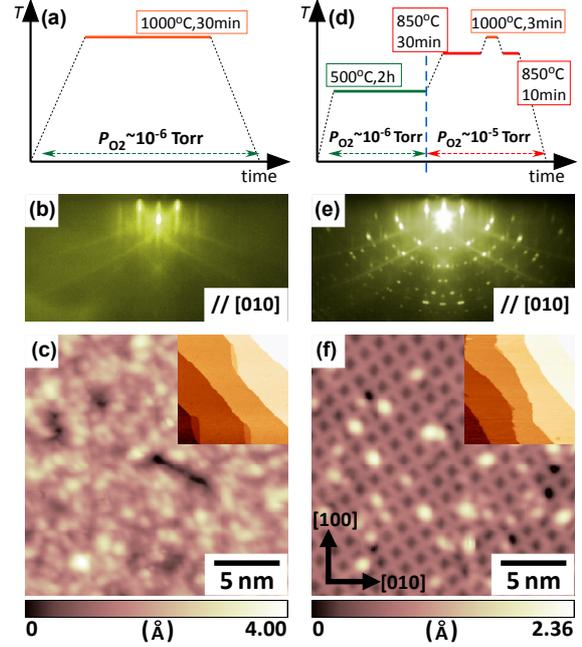
Figure 3: Schematic diagram of (a) typical and (d) new annealing processes. (b), (e): RHEED patterns (c), (f): STM images ( $20 \times 20 \text{ nm}^2$ ,  $V_s = +1.5 \text{ V}$ ,  $I_t = 30 \text{ pA}$  at  $77 \text{ K}$ ) on the surfaces annealed by process (a), (b), respectively. Insets show wide-view STM images ( $400 \times 400 \text{ nm}^2$ ,  $V_s = +2.0 \text{ V}$ ,  $I_t = 0.2 \text{ nA}$  at RT).
