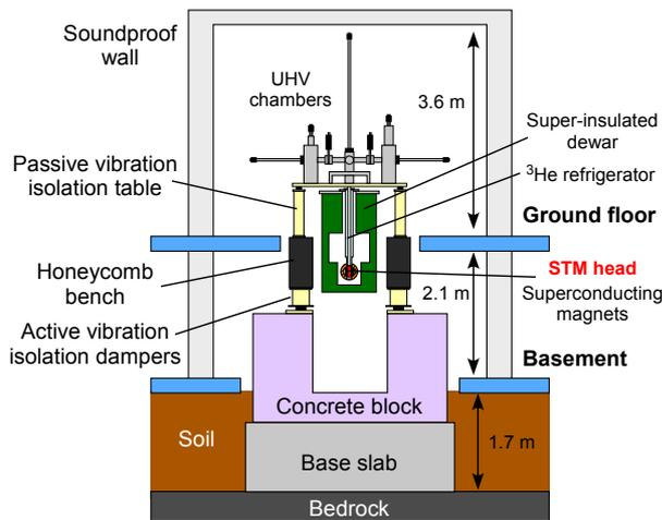
Figure 1: Schematic of newly-developed STM system.
