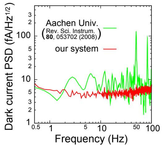
Figure 2: A fast-Fourier-transformed dark current noise spectrum with a reference one [2]. The preamplifier is the same as that of the reference.
