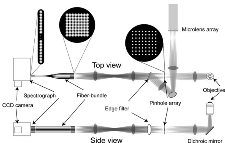
Fig. 2 Schematic of multi-focus confocal Raman microspectrometer
