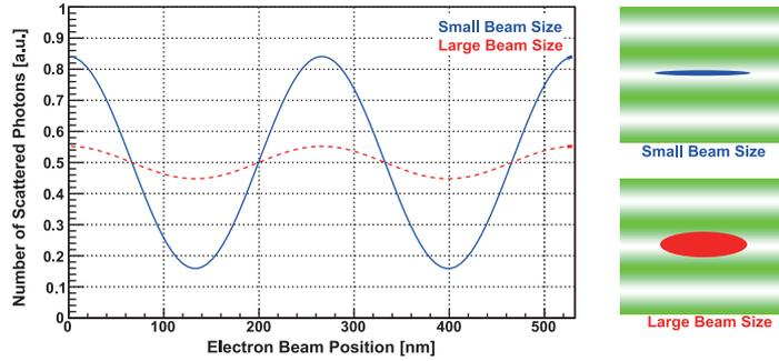
Figure 1: Different modulation for different beam size (from T.Suehara's doctor thesis)
