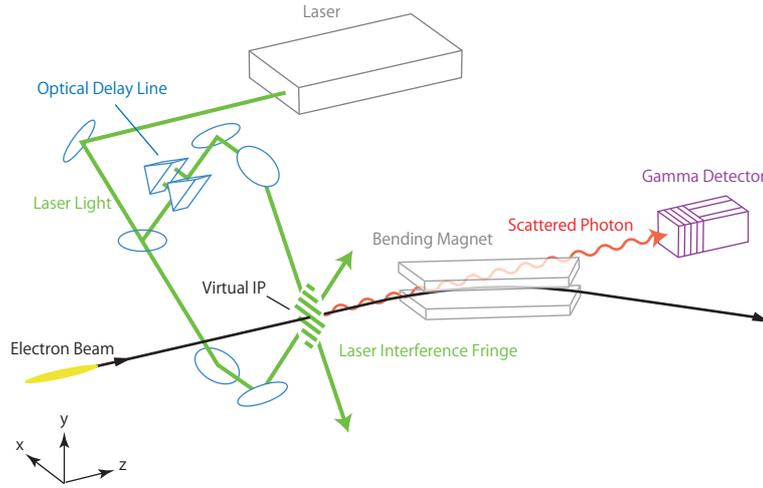
Figure 2: Schematic diagram of shintake-monitor at ATF2 (from Y.Yamaguchi's master thesis)
