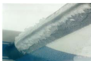
(Fig.2) In-flight icing on leading edge (1)
